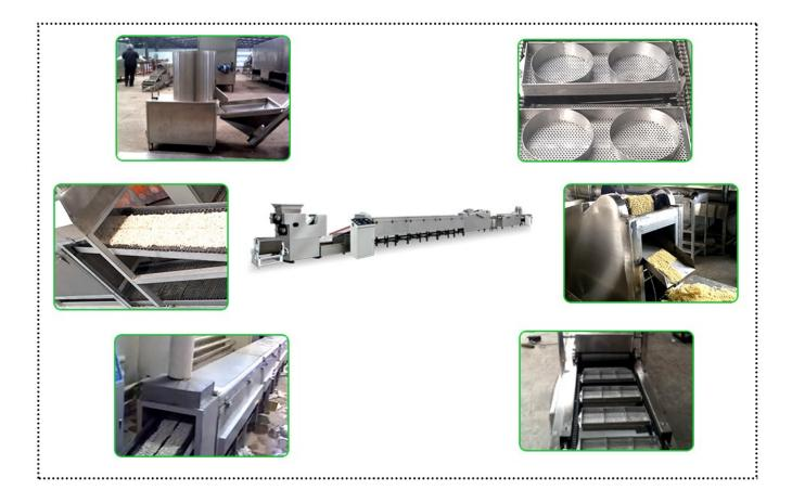
3. The oil must be added to the furnace body before the frying function is powered to avoid burning the electric heating tube;
