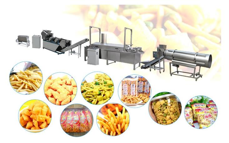
1. The fryer is composed of a mesh belt conveying system, a mesh belt lifting system, an automatic scraping system, an oil temperature control system, and a hot oil circulation system.
