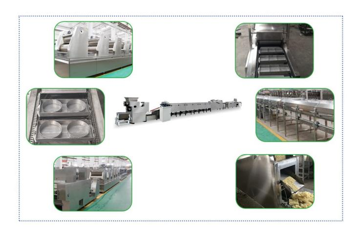
The instant noodles manufacturing process is, first of all, add 33% water to the flour. Use a kneading machine to reconcile the noodles, and then put the noodles into a calender to form a dough sheet. Then cut into noodles by a cutting machine. The cut noodles are sent to the steaming machine via a conveyor belt. Steam for 1-2 minutes, and then carry out the flavor treatment.
