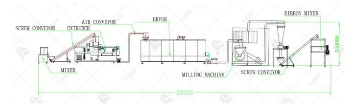
The mixer serves as the starting point of the entire production line, undertaking the crucial task of raw material pre-treatment. This device, through its special mixing mechanism, can thoroughly mix different raw materials with varying physical properties according to scientific ratios. Whether
