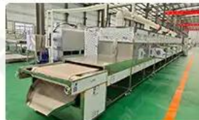
6. Machine Material : 304 stainless steel
