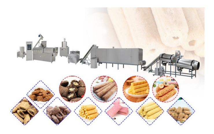
Automatic corn puffing machine belongs to a kind of equipment for processing puffed food, such as processing rice, corn, soybean, wheat and so on in daily life. Its main working principle is that mechanical energy is converted into heat energy. The heat generated when the machine rotates is used to squeeze and cook the food. The most obvious feature of the puffed snack is its larger volume.
