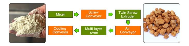
The technical key and focus of this production line is the use of extrusion technology. After the material is expanded, the volume will be enlarged, the taste will be crispy, the starch will be gelatinized, and the water-soluble components will increase, which is easy to be absorbed by the human body.
