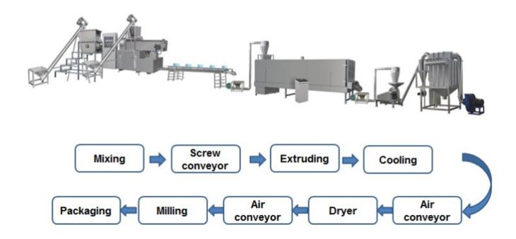
The baby food machine uses rice, corn, beans and various grains as raw materials. Through extrusion, expansion, drying, crushing and mixing, it can produce a variety of baby foods, such as baby rice flour, sesame paste, soy milk powder, nutritional powder, etc. The production line can automatically complete all processes from feeding to the end, with simple and convenient operation and high production efficiency.
