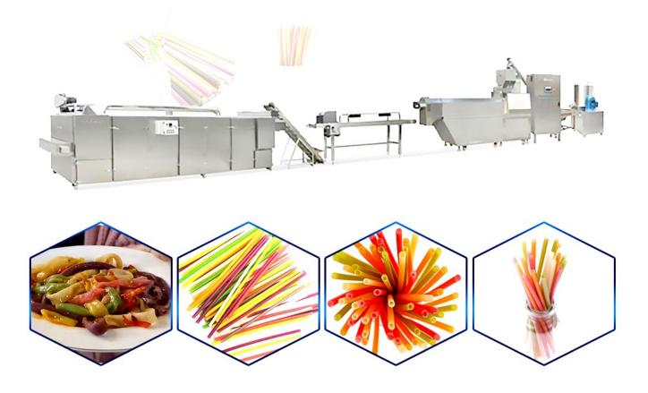
Edible straw production line is made into blanks of various sizes by a single screw extruder, and then dried to form straws with smooth surfaces and shapes. Our unit screw combination technology and the precise control of the production process allows you to have a wider choice of raw materials, higher product quality, and more variety. Single edible straw screw extruder
